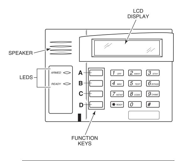
**IMPORTANT!:** When using the keypad to enter codes and commands, sequential key depressions must be made within 3 seconds of one another. If 3 seconds elapses without a key depression, the entry is aborted and must be repeated from its beginning.
